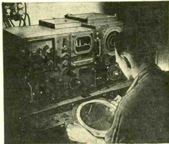
Photo 3—The Combat Information Center or control room on a flat-top carrier of the Essex class. A PPI (Plan Position Indicator) in use by a radar operator in this photo is being adjusted for signal pickup. The simple A scope can be seen just above his head to the left. A rack-and-panel set-up is employed in most of these installations.
